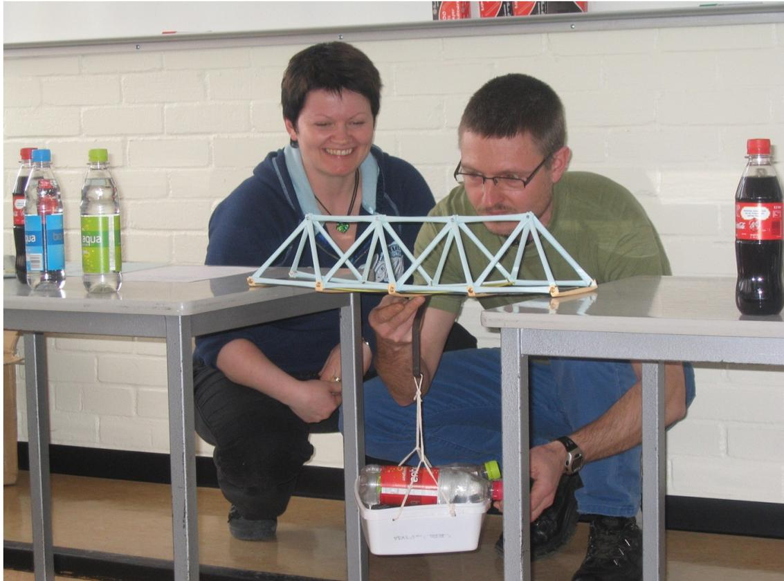
Teachers have built a bridge and are testing how much weight it can carry.
